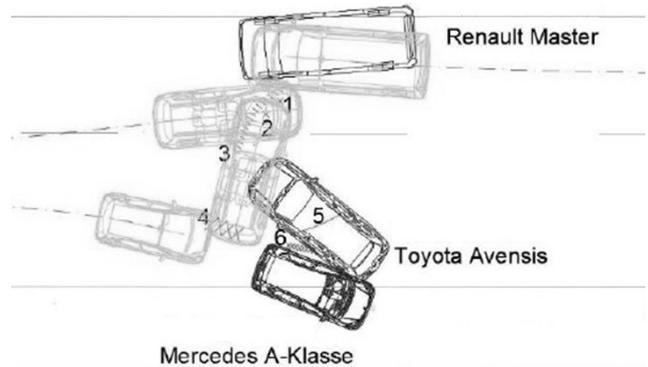
Figure 7. Accident site for a small overlap crash: maximum intrusion condition (light grey) and final (dark grey) positions are reported.
