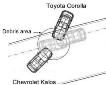
Figure 5. Frontal impact with maximum intrusion (light grey) and final (dark grey) positions of the involved vehicles.
