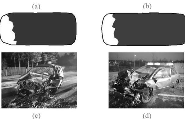
Figure 9. Reconstructed deformed shapes of the Chevrolet Kalos (a) and the Toyota Corolla (b) and the real ones (c,d).
