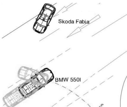
Figure 6. Side impact site with maximum intrusion condition (light grey) and final (dark grey) positions of the involved vehicles.
