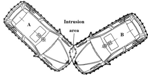
Figure 1. Two impacting vehicles with intruded nodes (light grey) and perimeters discretization in 50 elements each.
