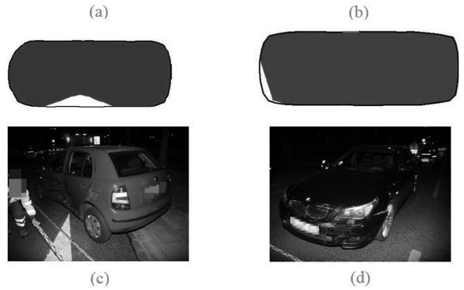
Figure 10. Reconstructed deformed shapes of the Skoda Fabia (a) and the BMW 550I (b) and the real ones (c,d).
