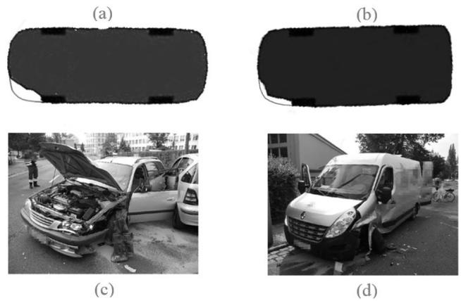
Figure 11. Comparison between reconstructed deformed shapes of the Toyota Avensis (a) and the Renault Master (b) with the real ones (c,d).
