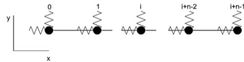
Figure 2. 1D representation of a vehicle's perimeter portion, with the nodes linked by springs to the virtual vehicle.
