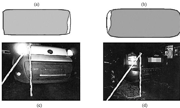
Figure 8. Reconstructed deformed shapes of the Fiat Fiorino (a) and the Audi A4 (b) and the real ones (c,d).
