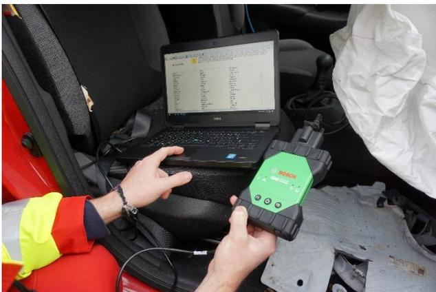
*Readout of an accident vehicle via OBD interface (incl. external power supply of the vehicle)*
