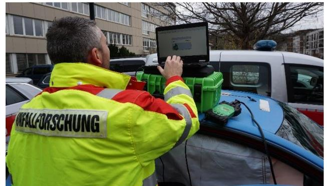
*Readout of an accident vehicle with the Bosch CDR 900 to obtain an EDR protocol*
